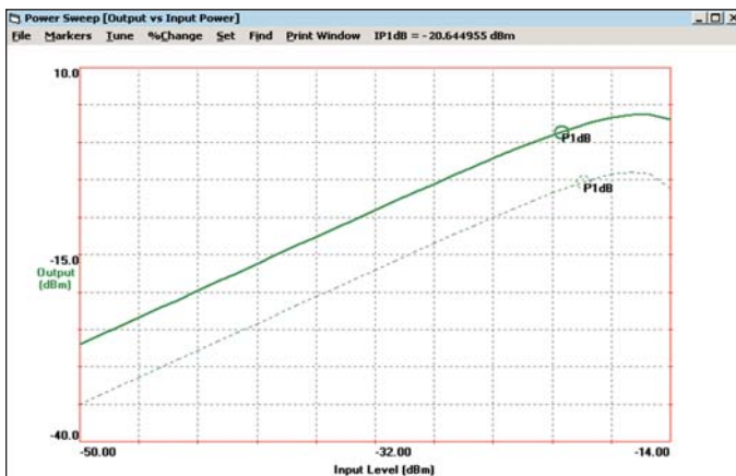
Figure 4 · The VSA’s power sweep plots.
